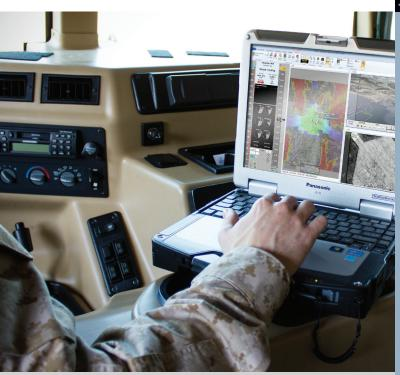
**Insitu's INEXA Control software application** builds on our proven unmanned experience to provide command and control of multiple UAVs and payloads from a single workstation, enhancing safe operation of our UAVs under the most demanding mission conditions.
