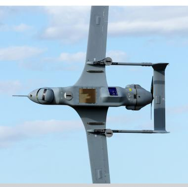
RedKite is a small electro-optical system capable of monitoring a city-sized area in real time. Simultaneously detects and tracks multiple geographically dispersed targets, allowing for in-flight forensic rewind and review.
