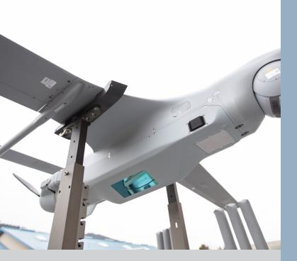
BlackKite streams geo-located imagery to multiple users for real-time and forensic analysis. The mid-wave infrared (MWIR) wide-area motion imagery (WAMI) system is capable of monitoring a city-sized area both day and night.
