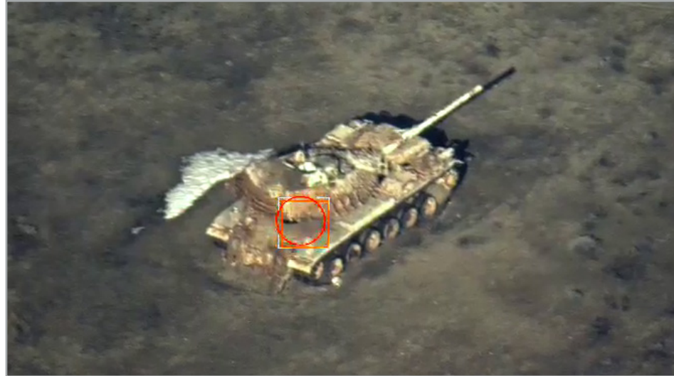
The laser spot tracker overlays a reticle on the video stream.
