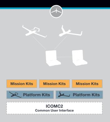
ICOMC2 is the common user interface for operation across Insitu's UAS platforms. The software supports customization using add-on kits for ultimate flexibility and expandability.
